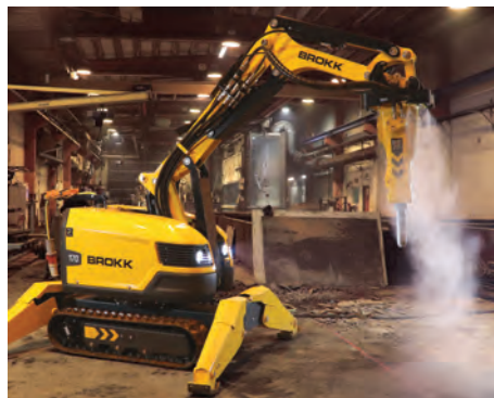
The Brokk Atomised Water Mist for dust suppression
